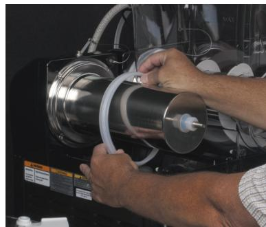
Step 5: Remove the hopper, auger, hopper seal, and auger nose seal, if used, from the machine. With the hopper removed you can now start disassembling the faucet assembly to be cleaned. Repeat the process for the other hopper. Remove the drip tray and grate to be cleaned with hopper parts. All items except for the rubber seals can be placed in the dishwasher. It is not recommended to use rinse agents if using the dishwasher- as this may cause stress cracking on the hopper.
