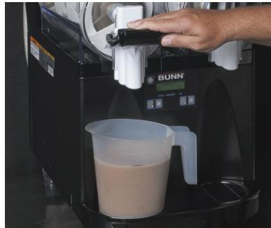
Step 3: Empty the product from the hopper. Try to get as much product out of the hopper as possible. Add warm water to help remove excess product if needed. All dispensed product must be thrown away and not reused. Repeat the process for the other hopper as necessary.
