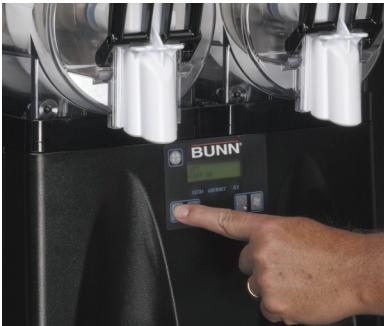
Step 1: In preparation for cleaning the machine turn-off the auto-fill function by pressing the "auger button" until the display reads "auger on". The auto-fill will need to be turned-off at a pre-determined period of time prior to cleaning. This will depend on your predicted volume thru the rest of the day.
