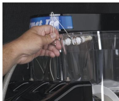
Step 8: Re-attach the auto-fill refill probe to the hopper. Then place the hopper lid back on-top of the hopper, plugging in the lid lamp. Re-connect the concentrate and water lines to the back of the hopper. Re-attach the drip tray and put the grate in place.
