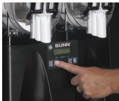
Step 9: Turn the auto-fill option back on by pressing the auger button until the display reads "left auger refill on". Followed by turning on the refrigeration by pressing the "snowflake button" until the display reads ice.
