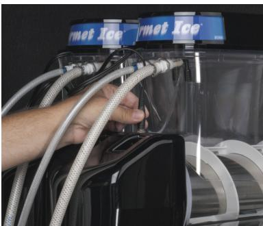
Step 4: Begin the hopper tear-down process by unplugging the lamp lid, followed by disconnecting the concentrate and water lines. Remove the hopper lid and set aside, this can not be submerged in water and must be hand-washed. Take-out the auto-fill refill probe, before you remove the hopper. Repeat the process for the other hopper.
