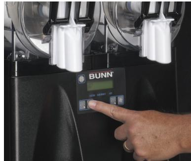
Step 2: When ready to begin cleaning, turn off the refrigeration by pressing the "snowflake button" until display reads off.
