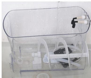
Step 6: If you are not using the dishwasher, place all removed and disassembled parts in the sink to be washed with warm soapy water. Once all parts have been washed place in a Kay-5 sanitation bath to soak for several minutes. While the parts are soaking wipe down the exterior of the machine, cooling drum, hopper drip tray, and auto-fill refill probe.
